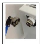
For a quick and thorough manual bleeding, open again entry and exit of the radiator and screw the venting hose (article number T2152) onto the air vent body mounted in the radiator.
