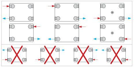
When connecting as a compact radiator, the valve insert has to be removed and plastic plugs have to be replaced with brass plugs.
